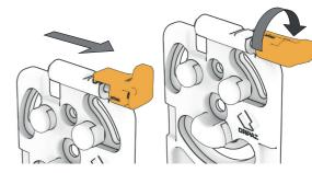
2. Align the insert with the receiver's locking holes (A) Slide the insert down until it stops in place.(B)
