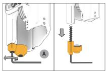
(**B**) Put the magnet aside, and keep the screw and spring.
