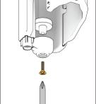
Insert the magnet into the sub compact extention, then connect everything together using the long Phillips screw.
