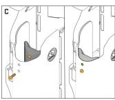
2. Once both pins are in place, and the spacer is stable, firmly hand tighten both screws.
